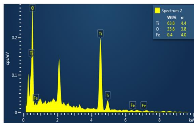
FIGURE 5. The map of EDS measurements: a) the map of different points taken the EDS, b) EDS spectrum of point 2
