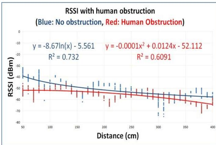
FIGURE 4: RSSI with human obstruction between the objects (after applying AOI with interval=60).
