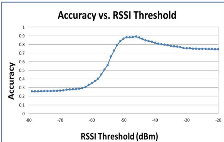
FIGURE 8: The accuracy of deciding if two Pi's are less than 2 meters apart given different RSSI thresholds after AOI filtering.
