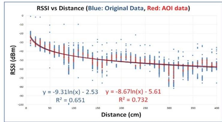
FIGURE 1: RSSI vs Distance, using raw data vs AOI data (interval=60).
