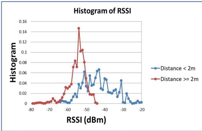
FIGURE 7: The histograms of RSSI when the distance is less than 2 meters or greater than 2 meters after AOI filtering.
