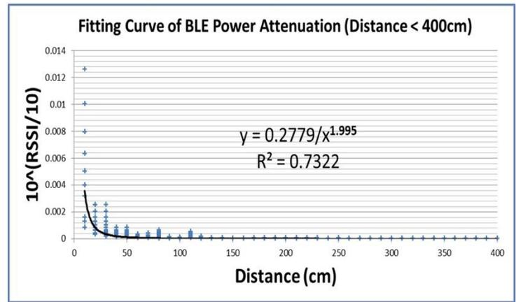
FIGURE 2: The fitting curve of BLE power attenuation after AOI.
