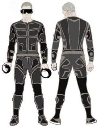
FIGURE 1: TESLASUIT is a full body haptic suit and training solution for physical VR experience. Author's own figure created in reference to TESLASUIT (2021).
