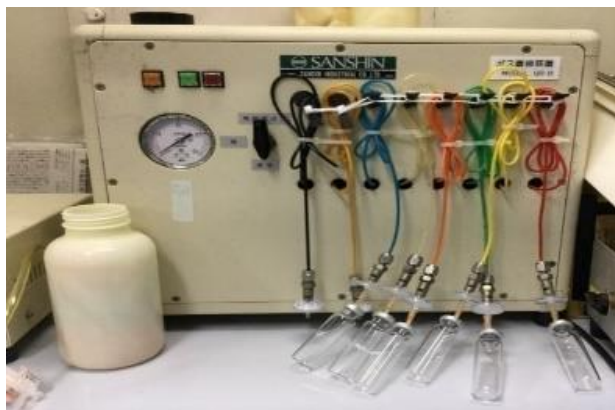
FIGURE 3. GAS EXCHANGE MACHINE DISPLACING OXYGEN GAS WITH CARBON DIOXIDE AND HYDROGEN GAS
