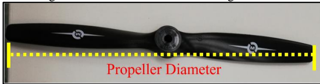
FIGURE 2 DESCRIPTION OF PROPELLER DIAMETER
